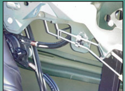
8. The cable of the power window mechanism is used to help position the tool.
